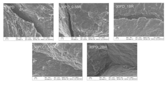
**Figure 2.** Cross-section morphology of CBFS without cross-linker (30PD), cross-linked CBFS (30PD\_0.5BR, 30PD\_1BR, 30PD\_1.5BR and 30PD\_2BR)
